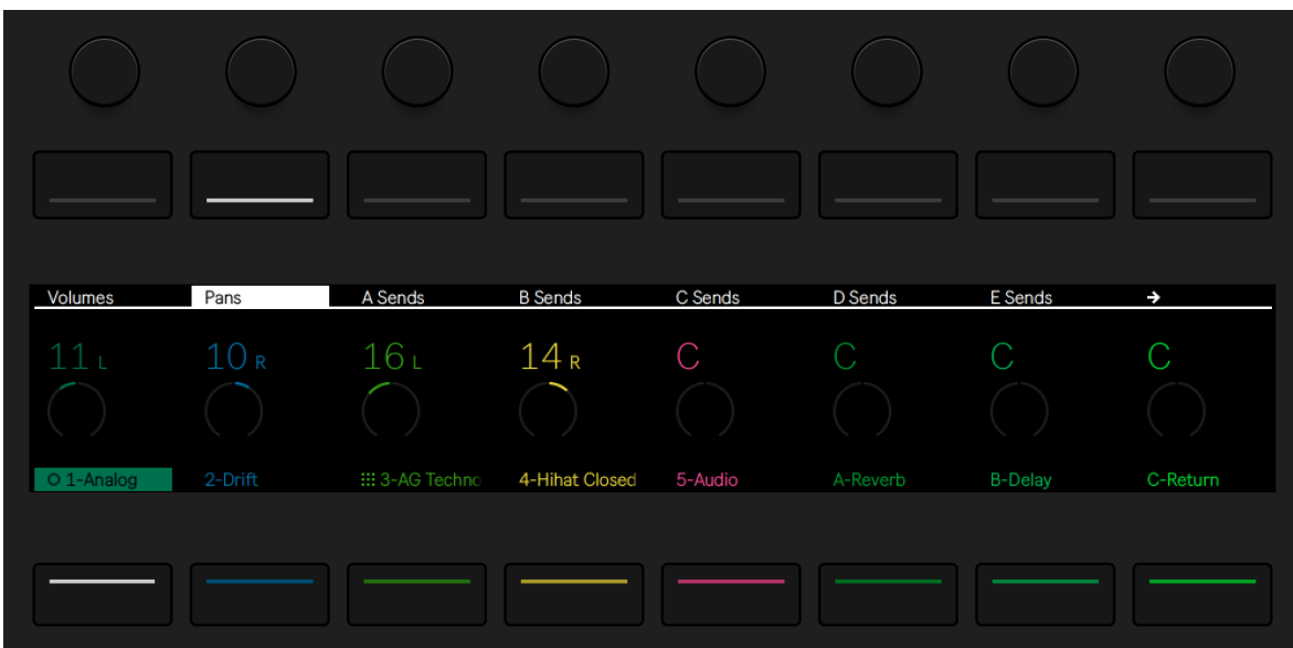
Controlling the Pans for Eight Tracks.
