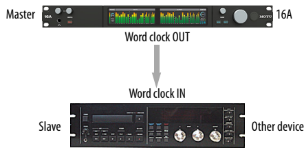
Figure 4-4: Slaving another digital audio device to the 16A via word clock. For the 16A clock source, choose Internal (or any source other than Word Clock , as daisy-chaining word clock is not recommended).
