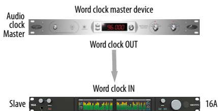
Figure 4-5: Slaving the 16A to word clock. For the 16A clock source, choose Word Clock In .
